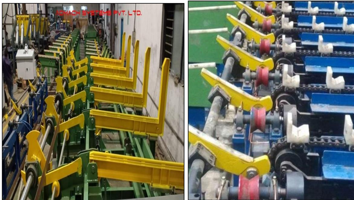
Bright bar handling systems are manufactured with special emphasis on smooth and scratch proof transportation of bars during various processes.
