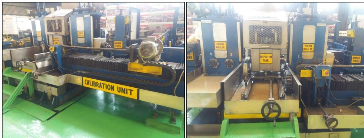
Black bar solutions involve handling and transporting less-processed iron bars, known as black bars, which are formed directly from raw iron. The black bar system is specifically designed to manage the movement of these bars from the station where they exit the moulding process, ensuring efficient and safe transfer within the production facility.
