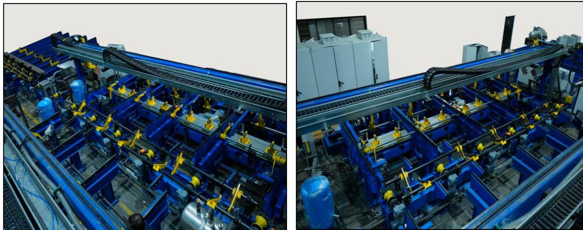
Bar MPI machines are crucial for identifying surface and subsurface defects in steel round bars and squares. These machines utilize magnetic particle testing to reveal flaws that may compromise the integrity of the material. MPI can be performed through visual inspection and manual marking or fully automated using advanced vision camera systems and artificial intelligence. This ensures precise detection and efficient quality control.
