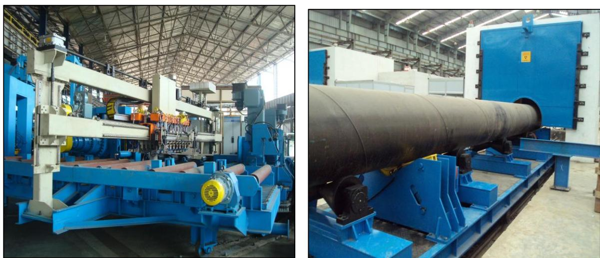
SAW (Submerged Arc Welded) pipes go through a specialized process to ensure top-notch quality and durability. The production includes X-ray and ultrasonic testing to inspect weld joints and pipe bodies. Pipes are thoroughly cleaned and inspected before protective coatings are applied. This integrated approach guarantees reliability for demanding pipeline applications.
