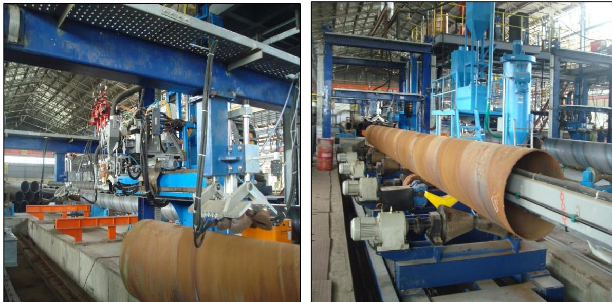
For faster production of pipes, they are tack welded on the forming mill and the final welding is done in offline mode. The offline welding stations do the internal as well as external welding of SAW pipes.
