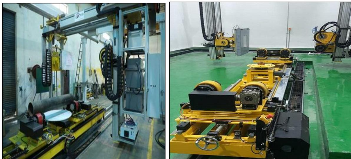
These are X-ray cabinets for special or bigger components. The flaws / porosities are detected in these machines.
