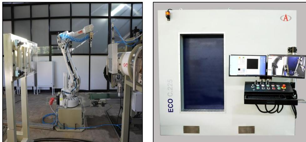
These are X-ray equipments for testing the forgings, castings, fuses and refractory materials. The entire test equipment with x-ray source and detector are enclosed in a lead shielded cabinet, so that the harmful radiations are not coming out. The flaws / porosities are detected in these machines.
