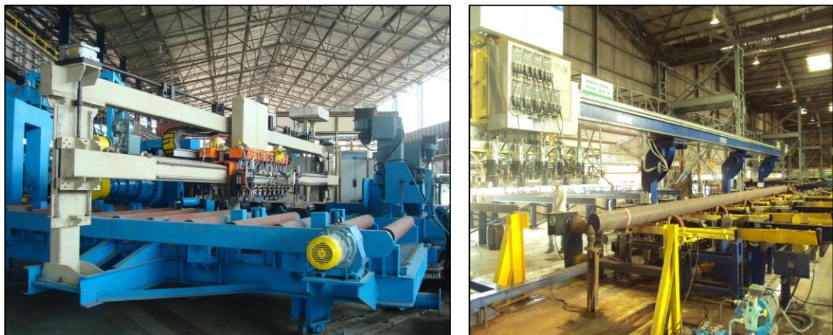
The ultrasonic testing is done for the weld joints of the pipe. These processes can be done in INLINE and OFFLINE mode. Also the coils (before forming the pipes) can be tested with an array of ultrasonic probes.
