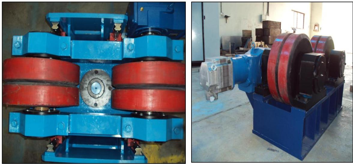
The SAW pipes are required to be rotated and lifted for conducting various processes. These are heavy duty equipments specially designed for taking care of heavy pipes.
