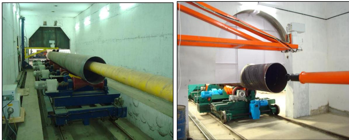
This is the X-ray process for the pipe testing which does the end tests as well as full pipe tests in the welded areas. includes conventional film-based methods, advanced digital techniques and SAW pipe cleaning.
