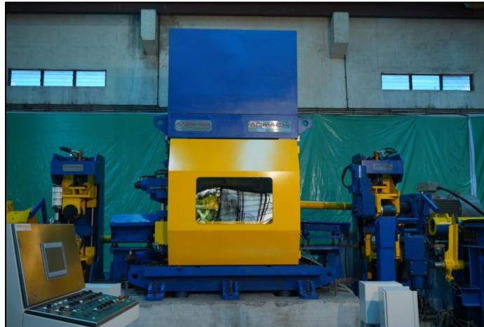
After the hot rolling process, alloy steel bars often become slightly curved or bent. This can cause problems during further processing and may not meet the quality standards of end customers. The bar 2-roll straightener is a machine that quickly and accurately straightens these bars. The straightened bars typically have a deviation of less than 1 millimeter per meter in length.
