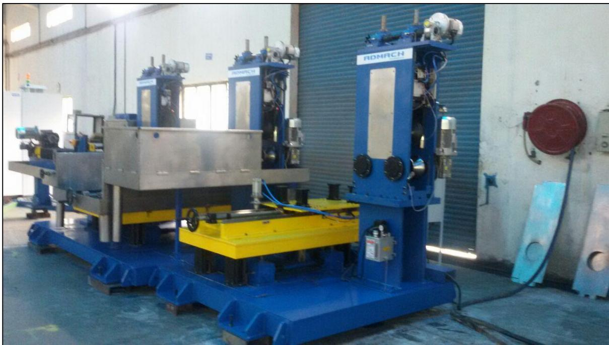
The steel bars are tested for these NDT processes. The MFL test is done for surface defect detection and the UT process takes care of the internal defects in the bars. Both these processes are conducted in INLINE mode and at a very high speed (up to 120 meters/minute).
