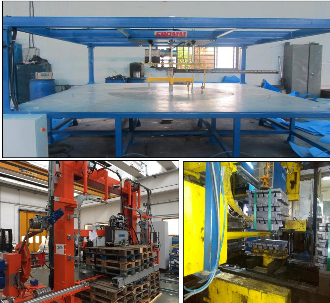
The steel bars, flats, coils, slit coils are packed using wrapping, strapping and taping processes. This is a very important process in the final product as it keeps the final product intact during transportation and inside shelves.
