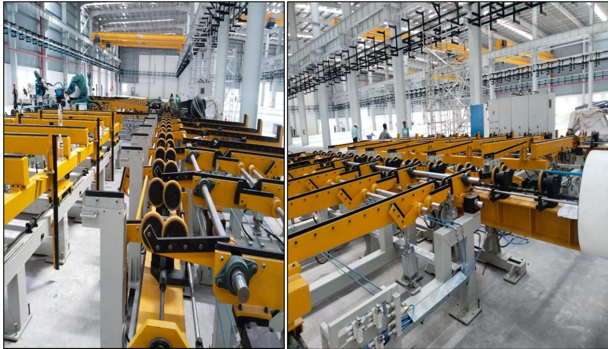
The bright (peeled) bars are ground in single and 2 passes to maintain size of the bar and also the surface finish of it.
