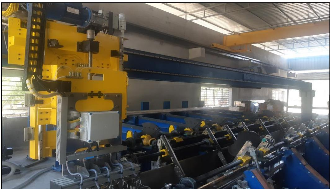
Bright bars are peeled bars where the skin of black bar is removed and the size tolerances are maintained, defects are checked with ultrasonic testing (UT). Finally, the finished bars are carefully packed to ensure quality is maintained.
