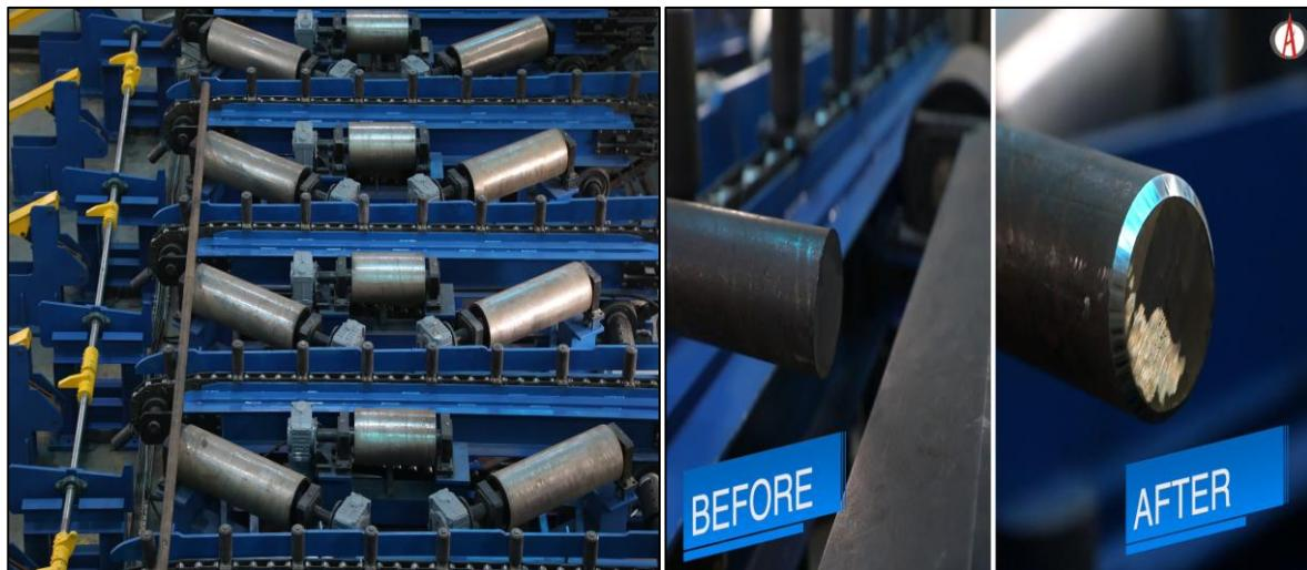
The bar end chamfering machine ensures that steel bars have smoothly chamfered edges. This prevents sharp corners from causing damage to equipment or injuries during subsequent processing and testing.
